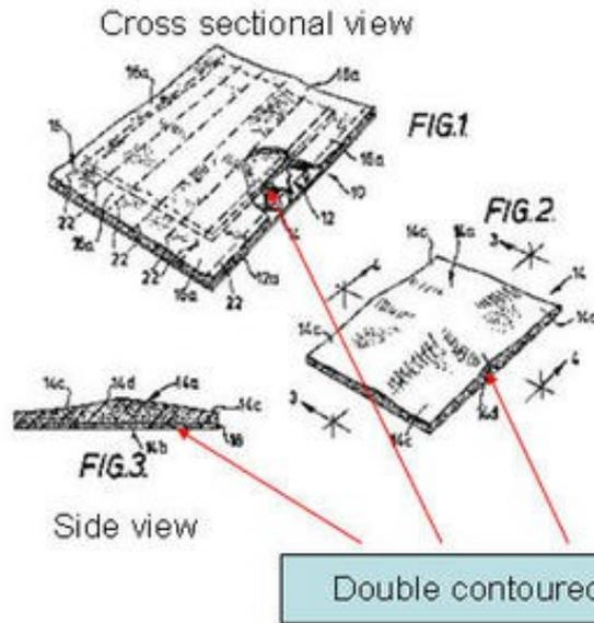
Double contoured batt layer of highly porous sandwiched between a porous facing layer and a water-impervious sheet. - High wettability and high fluid retentively
