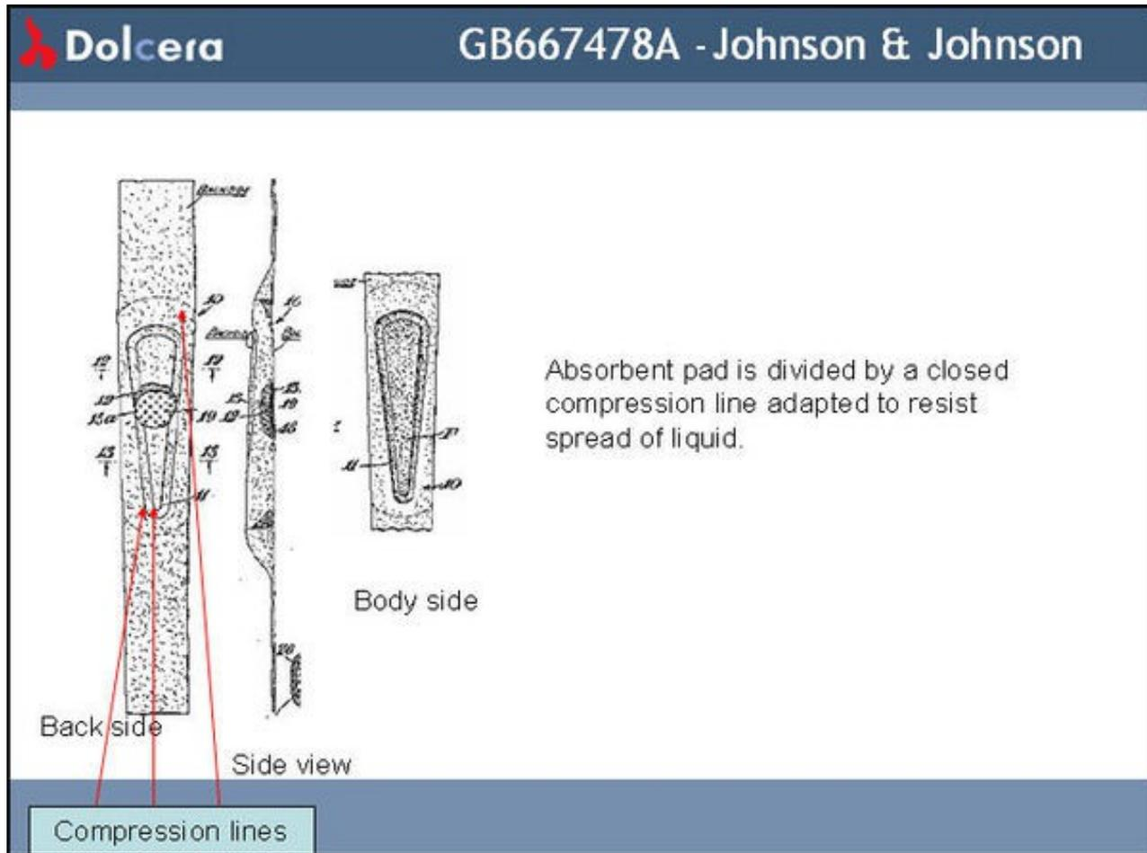
Absorbent pad is divided by a closed compression line adapted to resist spread of liquid.
