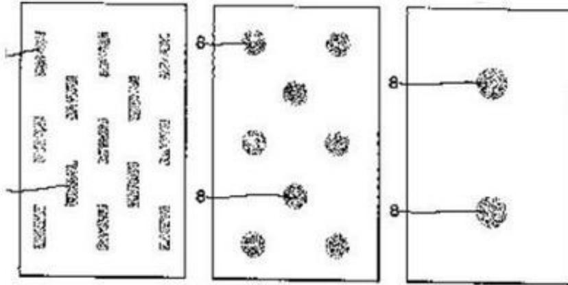
Alternative patterns for indicating agent (blue phthalocyanine dye and talcum powder) on absorbent pad - Indicates when to dispose diaper.
