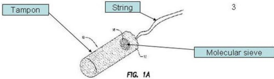
Molecular sieve (natural zeolite in powder form) disposed within the fibrous material to absorb odors from the body fluids.
