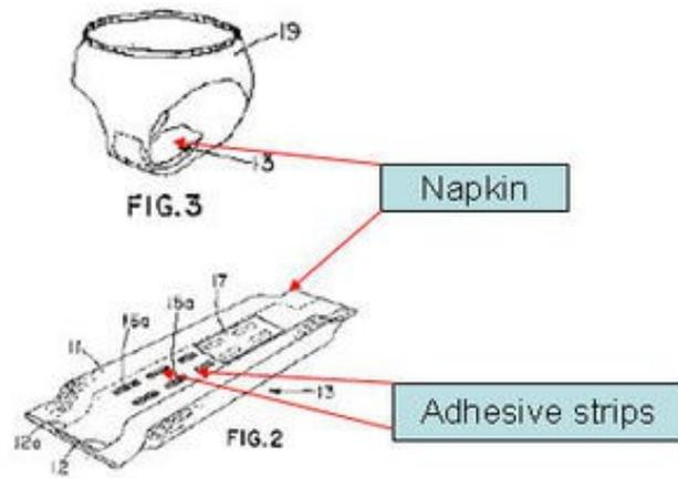
Two strips of adhesive extending longitudinally of the napkin is applied to the bottom side of the napkin. – For better attachment of napkin to garment
