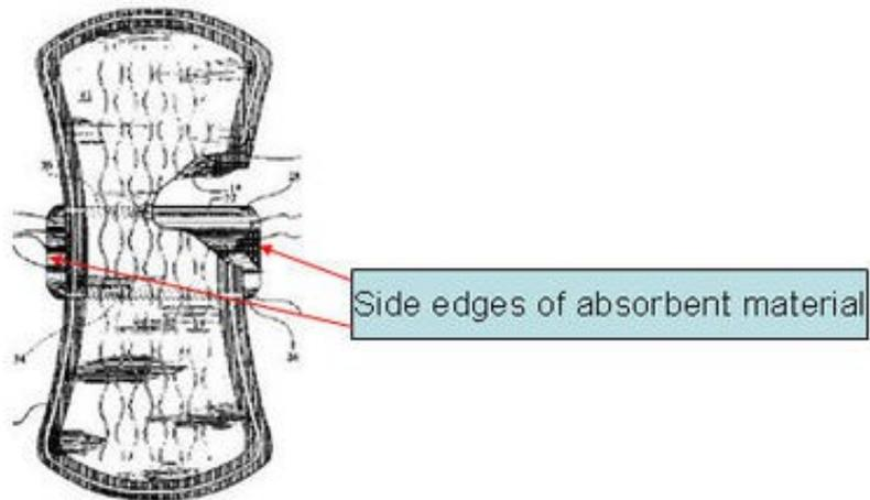
Structure having longitudinally extending side edges and transversely extending end portions (of absorbent material)
