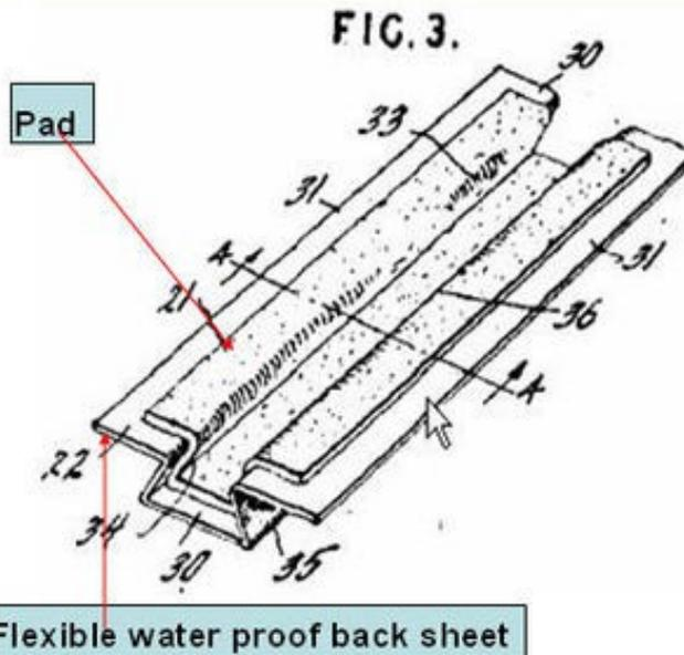
Diaper of rectangular form having flexible back sheet of waterproof material and a pad of absorbent material.
