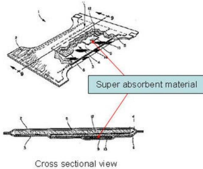
Super absorbent material (hydrocolloid materials) is sandwiched between two densified layers of cellulosic fiber - Enhances fluid distribution
