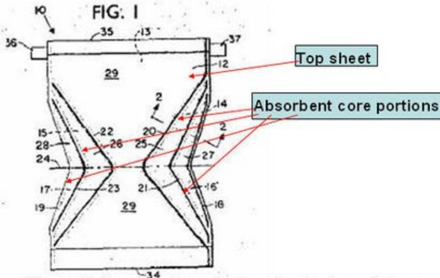
Diaper of **elongate shape** having absorbent core interposed between a moisture-permeable top sheet and a water impervious backing sheet.
