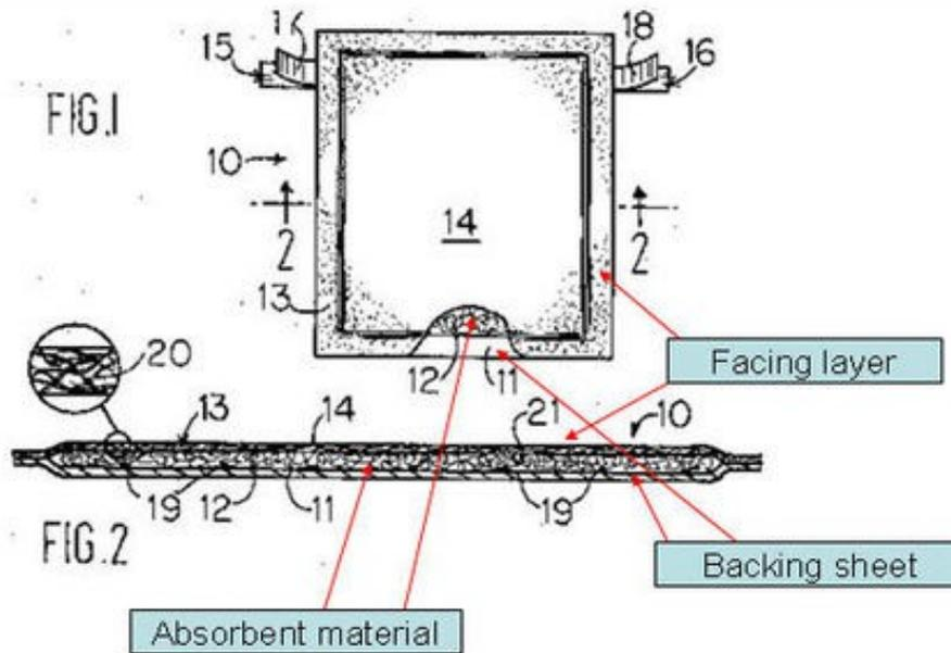
Fluid-impermeable backing sheet on which a layer of absorbent material is placed and a soft, body fluid-permeable facing sheet overlying said absorbent material - Soft feel, High absorption
