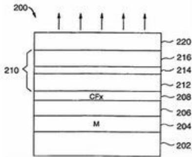
**Short summary:** The generated light is reflected at the mirror-like surface of the anode and transmitted through the cathode.
