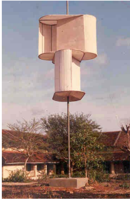
Fig. 2.7. A low cost Savonius wind turbine with rotors arranged 90^\circ out of phase
