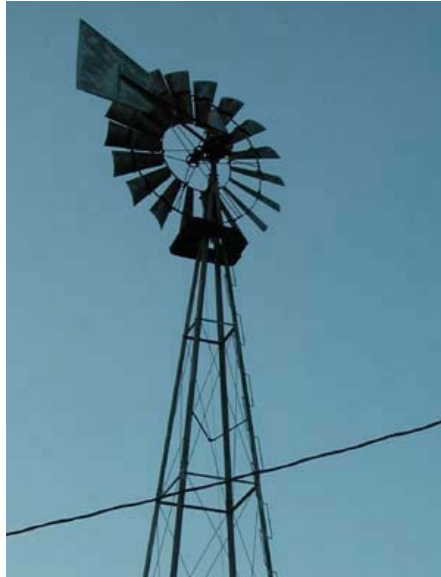
Fig. 4.29. A wind driven piston pump (Author: Pollinator, source: Wikipedia, http://wikipedia.org . GNU Free Documentation License applies to this image)
