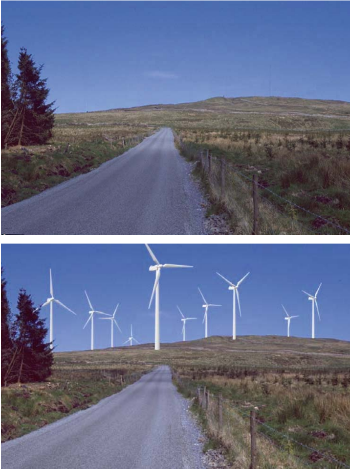
Fig. 6.9. Computer simulation of visual impact of wind turbines on landscape using the WindFarm Software ® (Courtesy of ReSoft, UK, www.resoft.co.uk )
