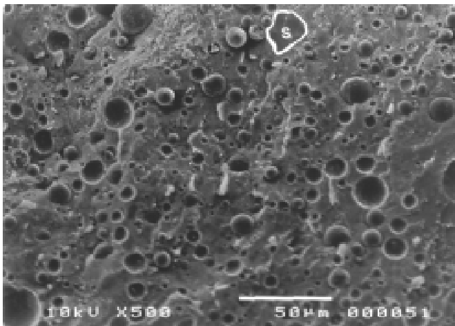
Figure 5—Electron micrograph (x 500) of imitation cheese containing 3% w/w native waxy-maize starch. S = starch particle (highlighted with a white border)
