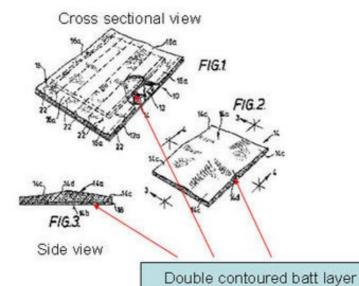
Double contoured batt layer of highly porous sandwiched between a porous facing layer and a water-impervious sheet. - High wettability and high fluid retentively
