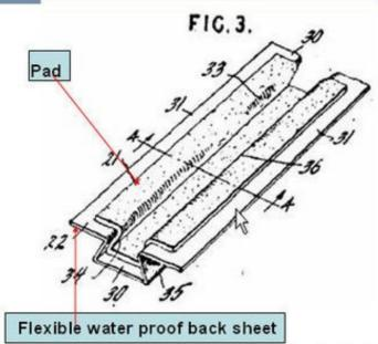
Diaper of **rectangular form** having flexible back sheet of waterproof material and a pad of absorbent material.
