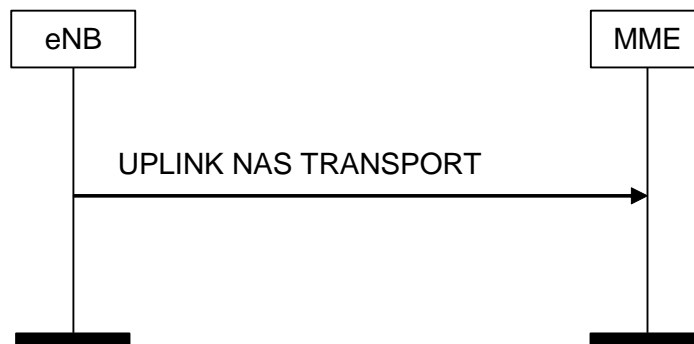
Figure 8.6.2.3-1: UPLINK NAS TRANSPORT Procedure
