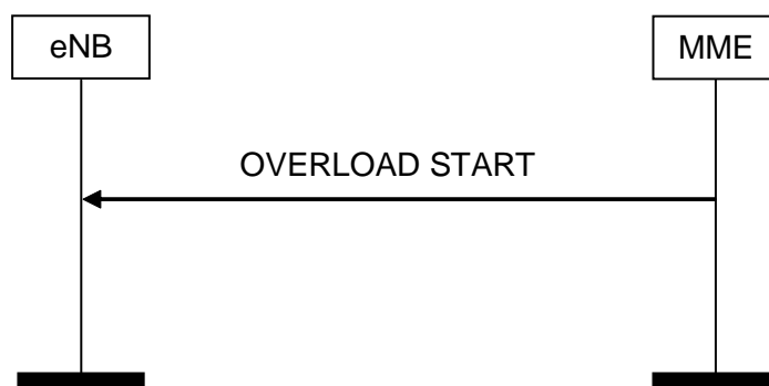
Figure 8.7.6.2-1: Overload Start procedure
