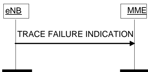
Figure 8.10.2.2-1: Trace Failure Indication procedure.
