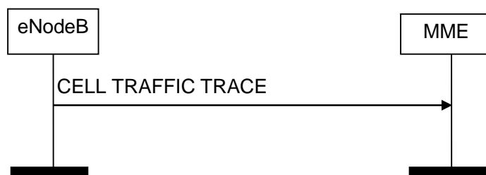
Figure 8.10.4.2-1: Cell Traffic Trace procedure. Successful operation.
