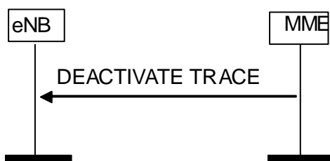
Figure 8.10.3.2-1: Deactivate Trace procedure. Successful operation.
