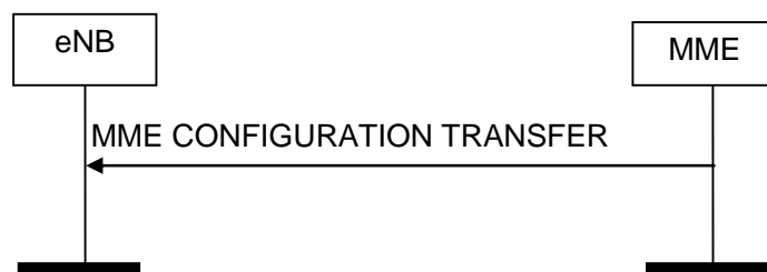
Figure 8.16.2.1-1: MME Configuration Transfer procedure. Successful operation.
