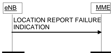
Figure 8.11.2.2-1: Location Report Failure Indication procedure.
