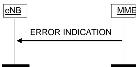
Figure 8.7.2.2-1: Error Indication procedure, MME originated. Successful operation.
