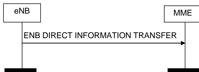
Figure 8.13.1.2-1: ENB Direct Information Transfer procedure. Successful operation.
