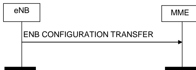
Figure 8.15.2.1-1: eNB Configuration Transfer procedure. Successful operation.
