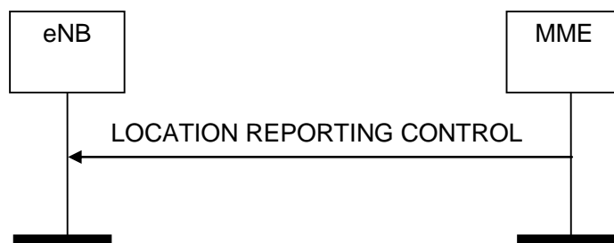
Figure 8.11.1.2-1: Location Reporting Control procedure. Successful operation.
