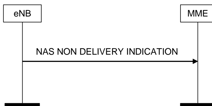
Figure 8.6.2.4-1: NAS NON DELIVERY INDICATION Procedure
