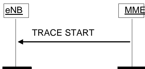
Figure 8.10.1.2-1: Trace Start procedure.
