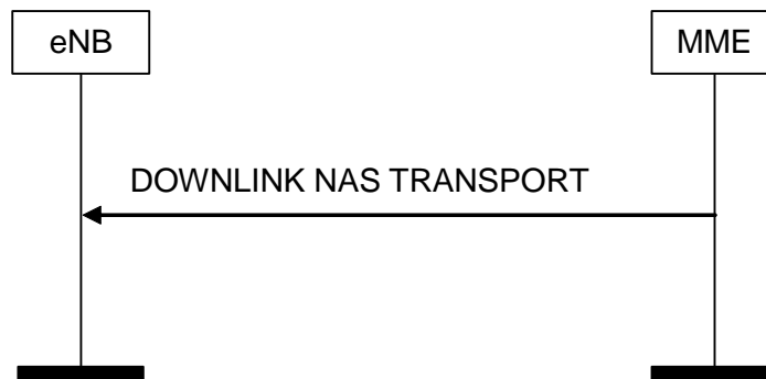
Figure 8.6.2.2-1: DOWNLINK NAS Transport Procedure
