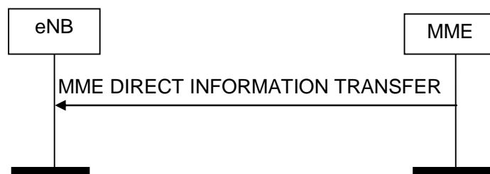
Figure 8.14.1.2-1: MME Direct Information Transfer procedure. Successful operation.
