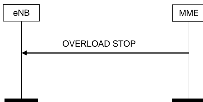
Figure 8.7.7.2-1: Overload Stop procedure
